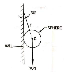
Calculate Tension produced in strings for the figure as shown below.
